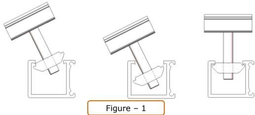
5.2.1 Assemble the earthing clip under the end clamp, then tilt the rail nut of end lamp into mini rail channel. Place the first panel on the mini rail and fix it with end clamp and earthing clip. The pins of earthing clip should penetrate both panel frame and mini rail.
