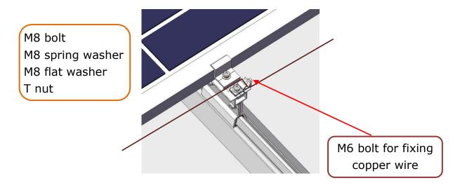
5.3.2 Connect each panel arrays by the copper wire through grounding lugs and tighten the M6x16 bolt.
