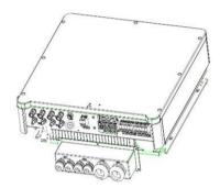
3) Step3. Disassemble the waterproof connector and pass the cable through the waterproof connector.
