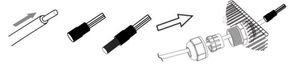
4) Step4. Connect the AC connector to the GRID port of the inverter with a slotted screwdriver
