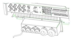
5) Step5. Assemble waterproof connectors and waterproof covers plate.
