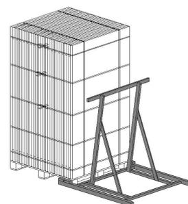
Place a support bracket on either of the recline surfaces of the assembly and remove the three transverse steel strips from the upper part of the assembly with
