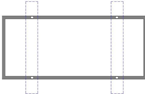
Installation rail vertical to the long side of the module, applicable type:
