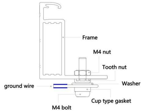
Figure 2. Grounding method
