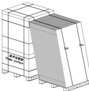
Gently push the module so that it leans against the support, removing the vertical strip of plastic steel
