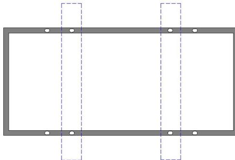
Installation rail vertical to the long side of the module, applicable type:
