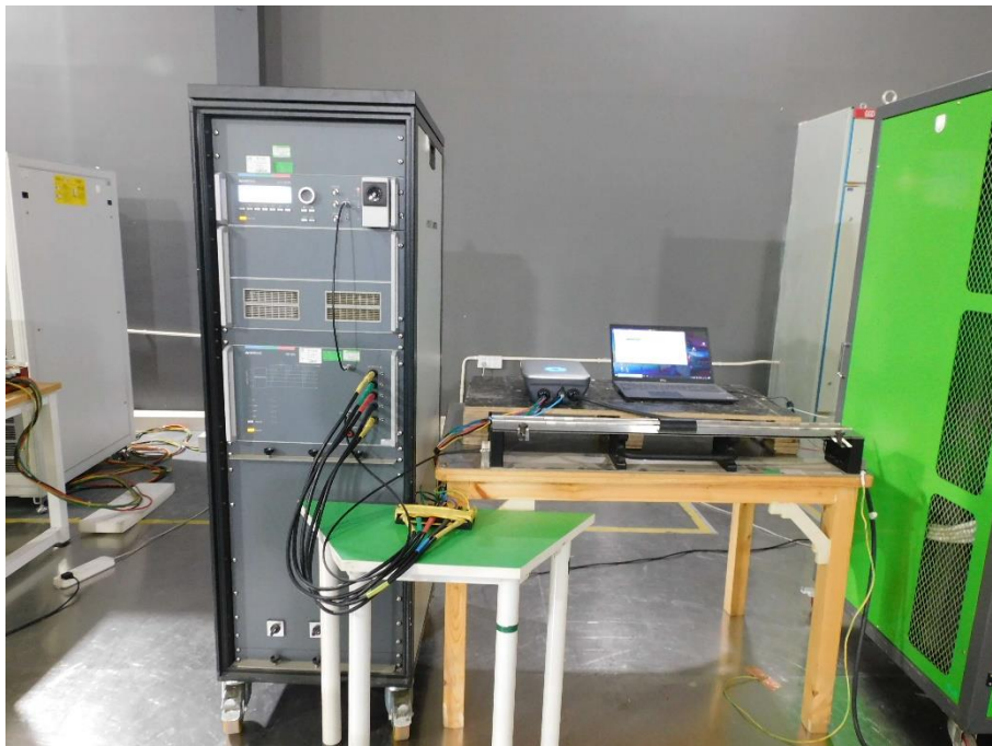
Photograph 10: Set-up for Electrical Fast Transients (EFT), Signal Port
