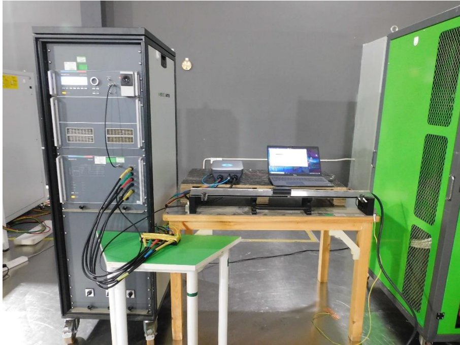
Photograph 11: Set-up for Electrical Fast Transients (EFT), CPT Ports
