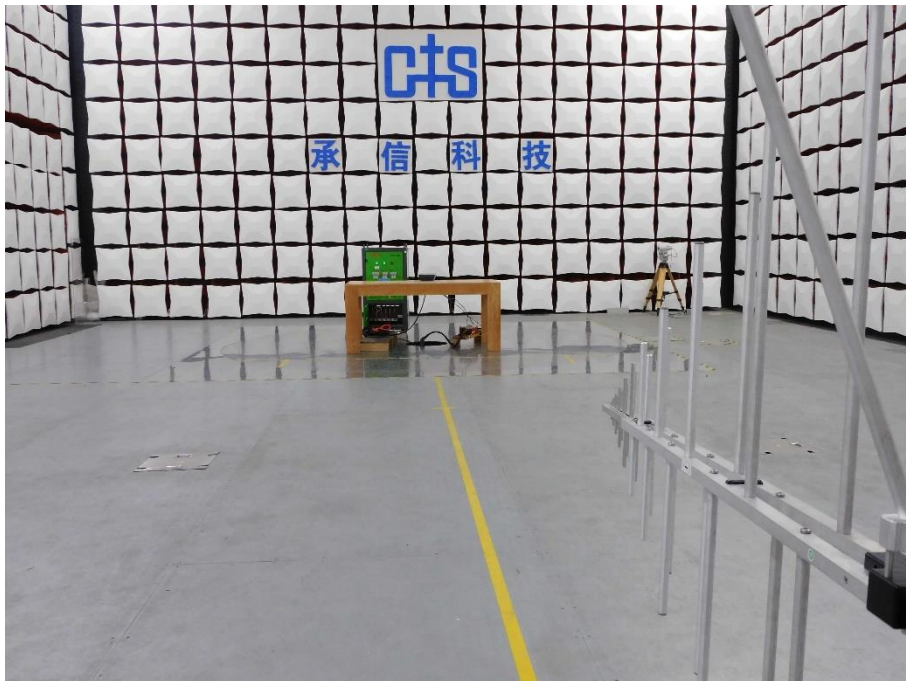
Photograph 2: Set-up for Radiated Emission, Below 1GHz
