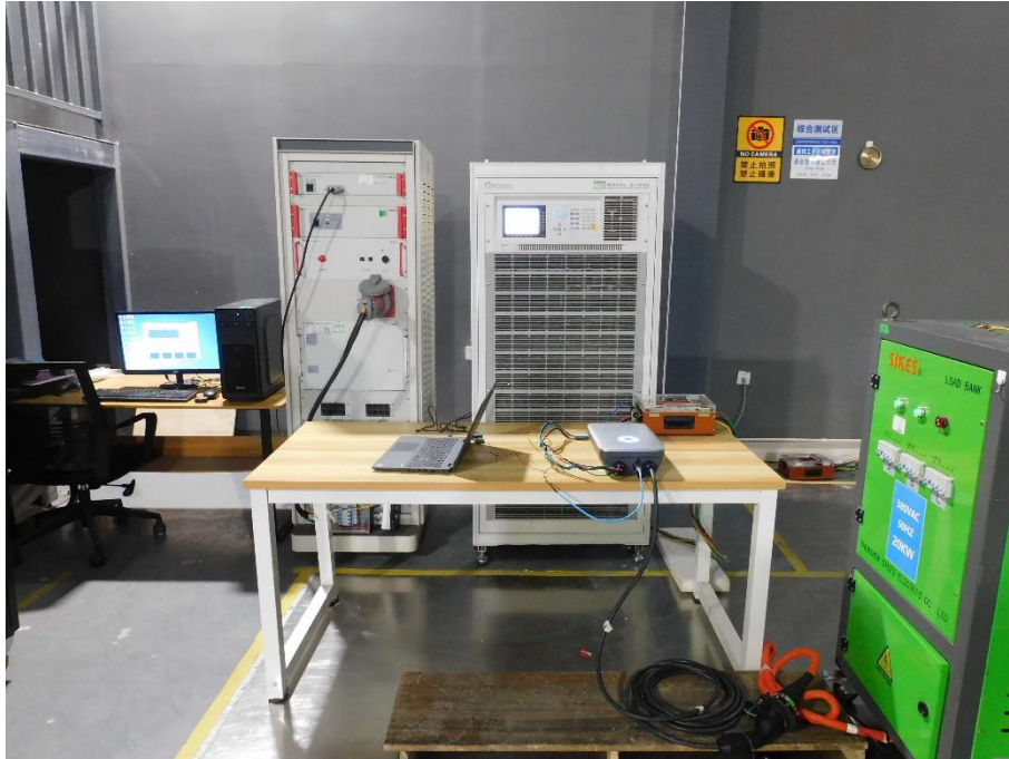
Photograph 17: Set-up for Voltage Dips and Interruptions
