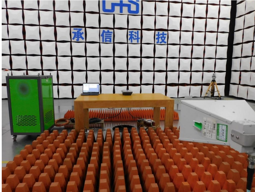
Photograph 3: Set-up for Radiated Emission, Above 1GHz
