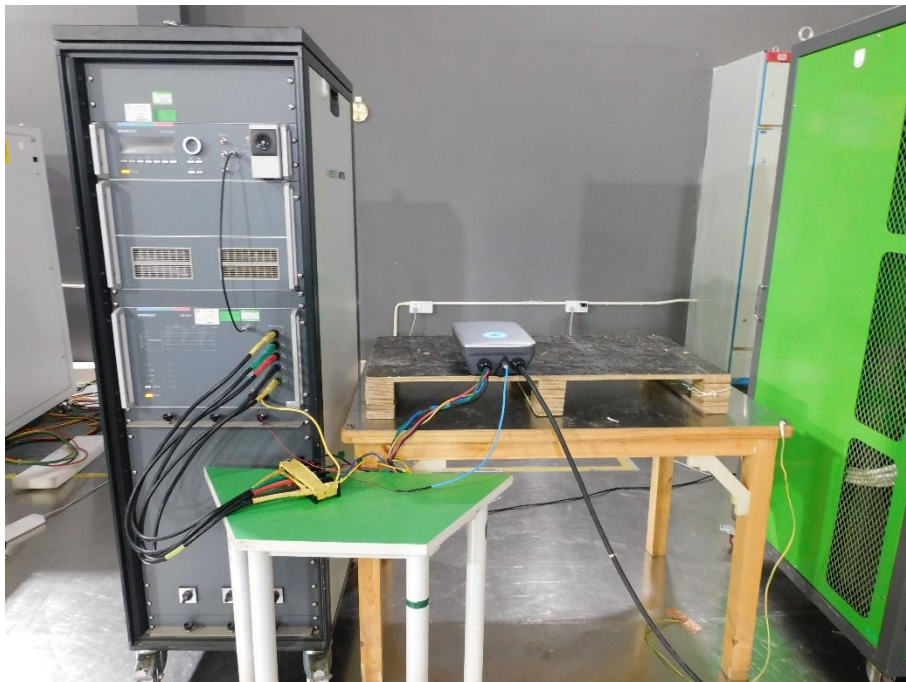
Photograph 16: Set-up for Surge, Signal Port
