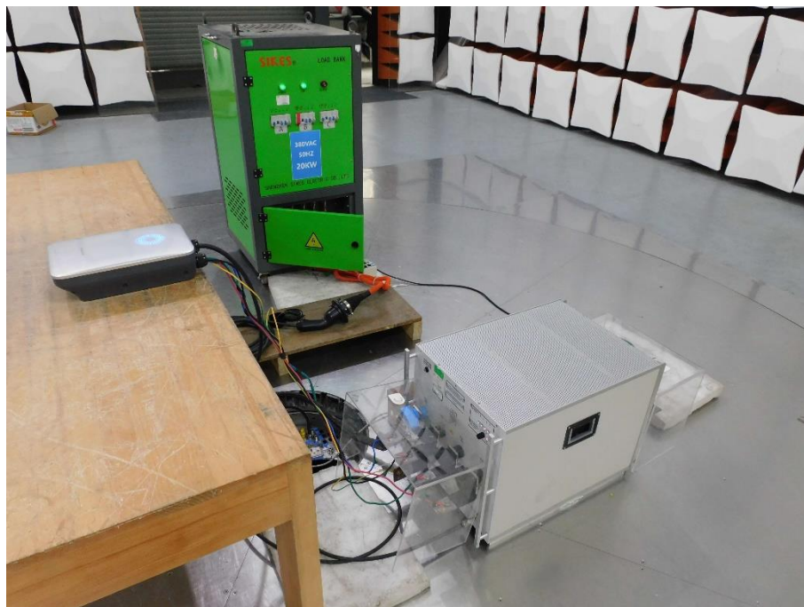
Photograph 4: Set-up for Conducted Emission, AC Mains Port
