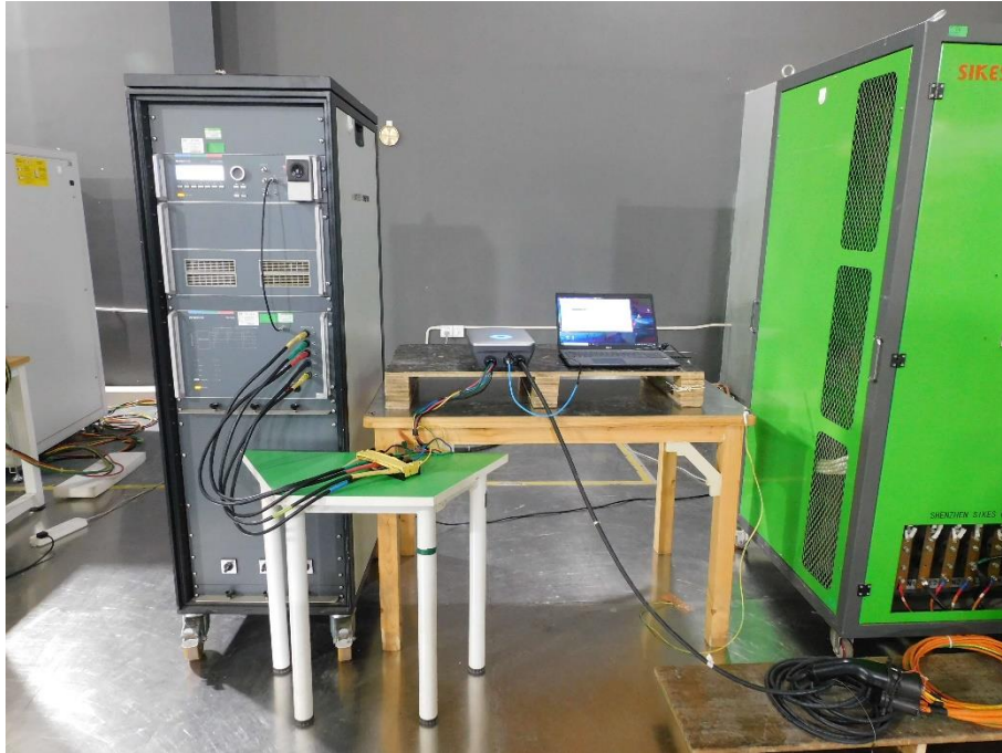
Photograph 9: Set-up for Electrical Fast Transients (EFT), AC Mains Port
