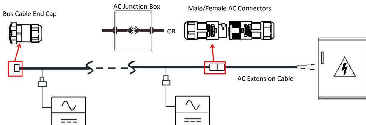
When AC extension cable is needed, users could connect the AC bus cable and AC extension cable in a junction box or use a pair of male/female AC connectors that APsystems provides as optional accessory.
