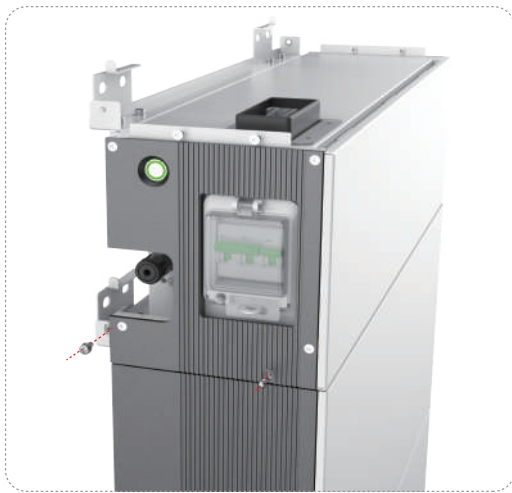
Figure 3-4 Left side screw installation
